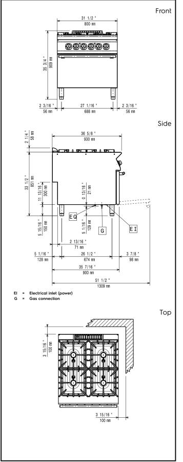
Modular Cooking Range Line 900XP 4-Burner Gas Range on Electric Oven
